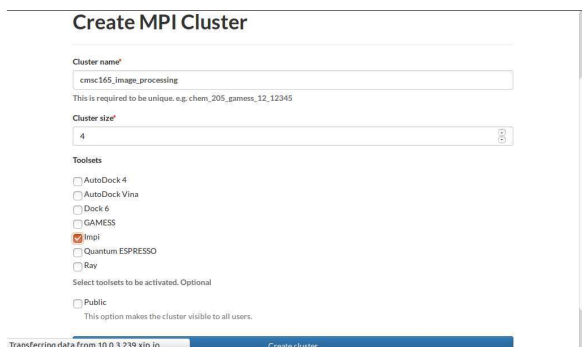
Figure 4: MPI cluster creation. A cluster named cm5c165_image_processing is being created with the Impi tool checked to be activated.
