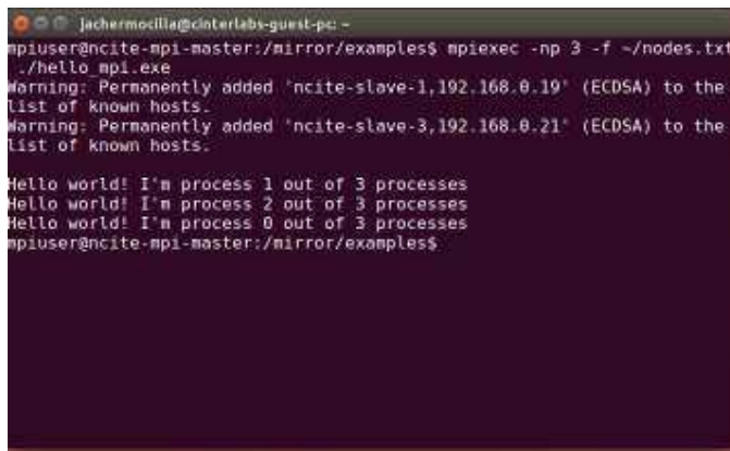
Figure 3: A hello world application running on a virtual MPI cluster deployed on P2C.
