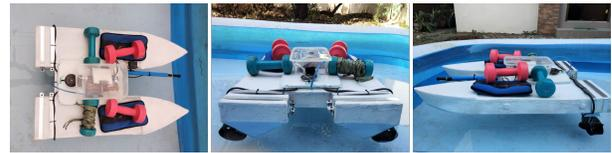
Figure 10: The ASV carrying an additional 11.1 kg load on its deck.
