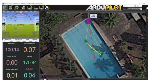
**Figure 15: Mission Planner view of the mission performed by the ASV in UPLB Baker Hall pool.**
